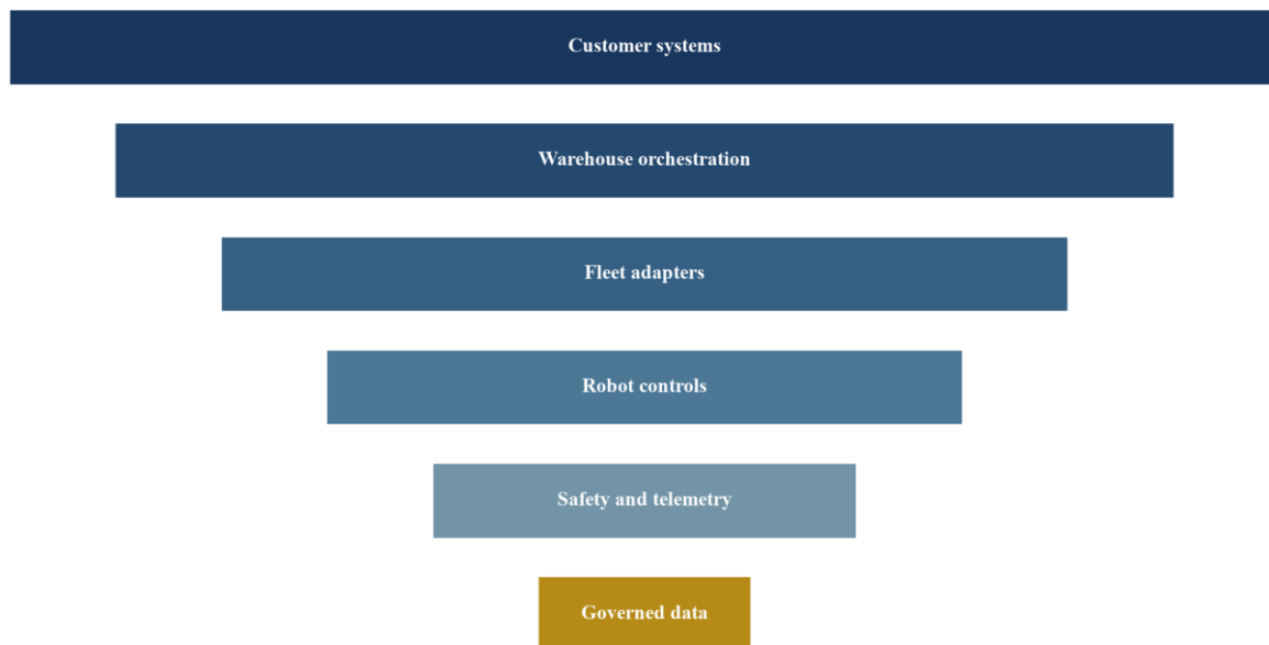
Figure 2. Layered mixed-fleet interoperability architecture
