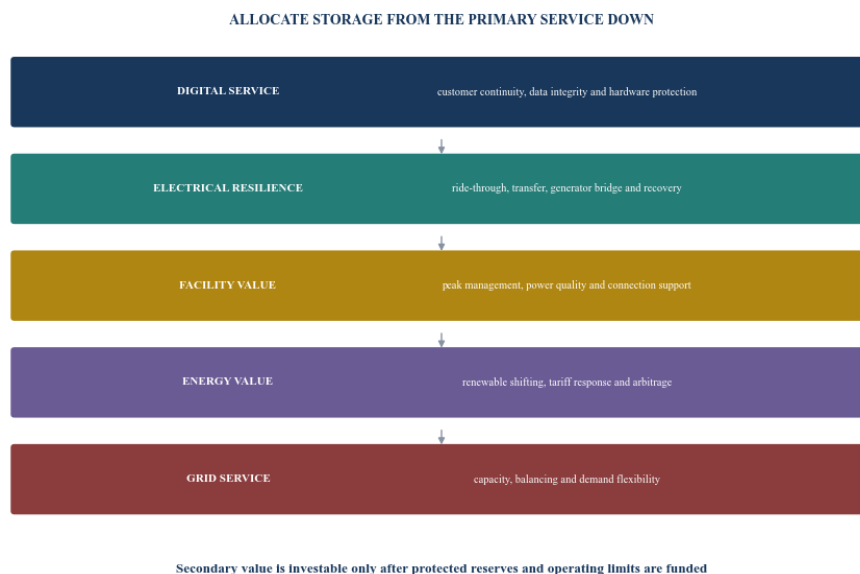
Figure 1. Battery service hierarchy beside a data centre
