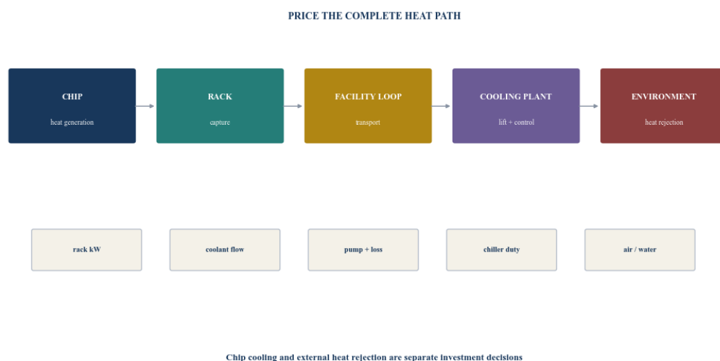
Figure 1. Heat path from compute to the environment
