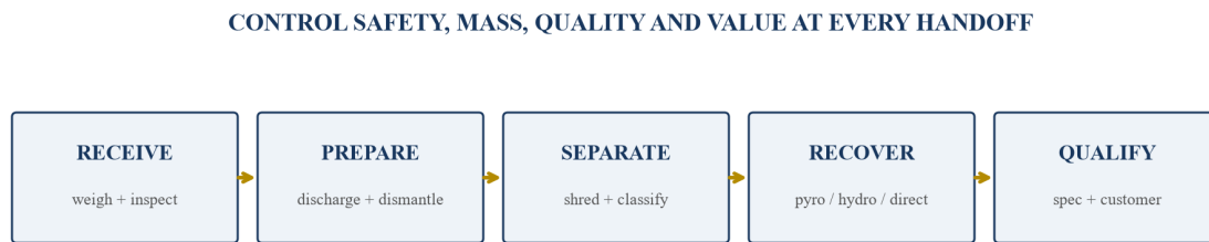
Figure 2. Battery-recycling process and value chain
